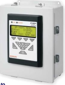
The AF-900PC Air/Fuel Ratio Control System utilizes heated O2 sensors and full-authority fuel valve control to precisely maintain the air/fuel ratio of rich-burn carbureted gaseous fueled engines.
